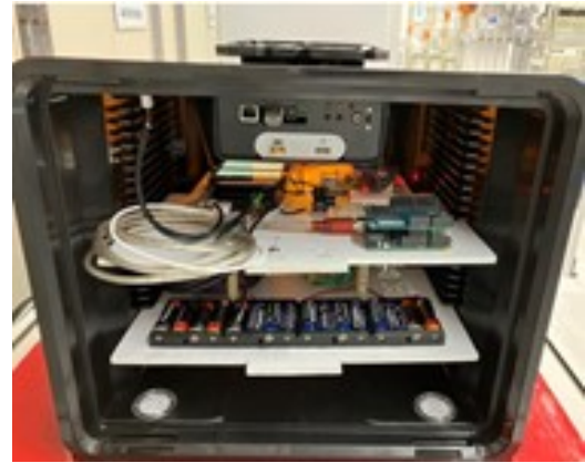
(b) Sensor platform in a FOUP
