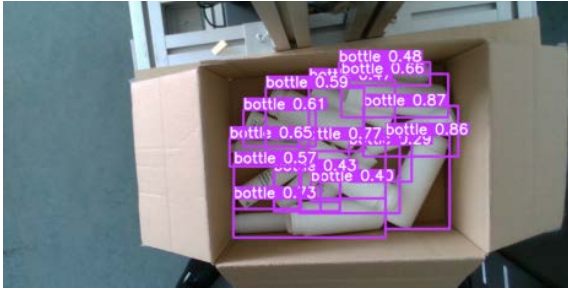
(a) Object detection results for the bottle objects (RT-DETR)
