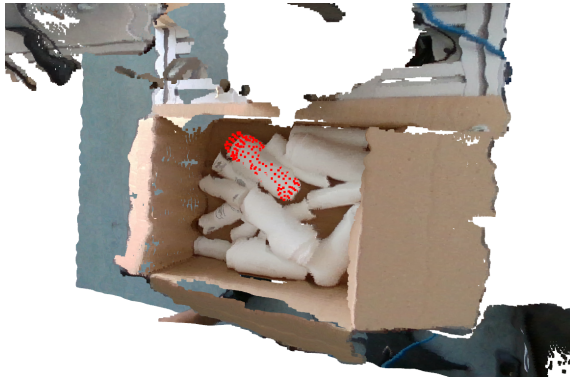
Fig. 3. The result of the point cloud fitting using ICP algorithm for one of the bottles
