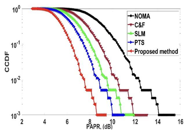
Fig. 4. PAPR analysis of 512 sub-carriers for NOMA waveform
