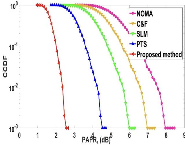
Fig. 2. PAPR analysis of 64 sub-carriers for NOMA waveform
