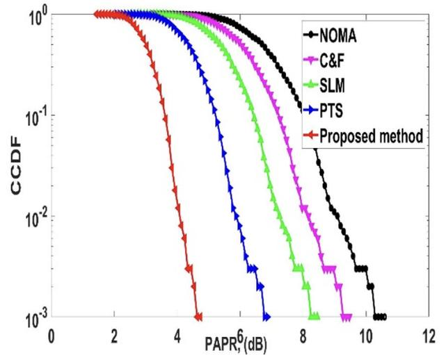
Fig. 3. PAPR analysis of 256 sub-carriers for NOMA waveform
