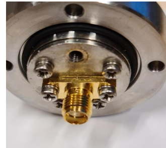
Fig. 9. Coaxial SMA connector attached to the circular waveguide
